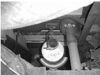
INSTALL MUFFLER ONTO HEADPIPES NO MORE THAN 1 1/2" TO 2" USING CLAMPS #G. USE A JACKSTAND TO SUPPORT MUFFLER.
