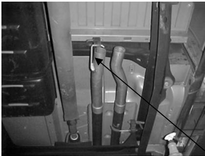
CUT YOUR STOCK HEADPIPES 17" IN FRONT OF STOCK MUFFLER USING A HACKSAW AND REMOVE STOCK EXHAUST SYSTEM. LEAVE FACTORY RUBBER GROMMETS IN PLACE.
