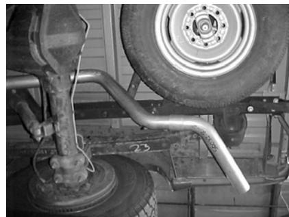
INSERT TURNOUT PIPE #E ONTO TAILPIPE AND ROTATE FOR YOUR DESIRED LOOK. USE CLAMP #H TO CONNECT TAILPIPE AND TURNOUT PIPE TOGETHER. DO NOT TIGHTEN.
