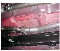
BOLT HEADPIPE #A TO THE STOCK FLANGE RE-USING THE FACTORY NUTS & BOLTS. INSERT WELDED HANGER INTO RUBBER GROMMET.
