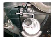
Next install rear muffler hanger #F onto outlet of the muffler. Insert hanger into rubber grommet. Do not tighten
