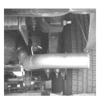
INSTALL EXIT PIPE #D ONTO OVERAXLE TAILPIPE USING CLAMP# E TO SECURE. ROTATE EXIT PIPE UNTIL IT IS AT THE CORRECT ANGLE FOR YOUR TRUCK. INSERT WELDED HANGER INTO RUBBER GROMMET.
