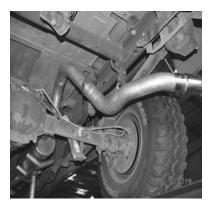
INSTALL OVERAXLE TAILPIPE #C INTO THE OUTLET OF THE MUFFLER 1 ½" TO 2" USING CLAMP #E TO SECURE PIPE TO MUFFLER. INSERT WELDED HANGER INTO RUBBER GROMMET.
