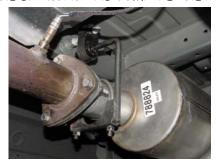
ATTACH FRONT MUFFLER HANGER #B TO MUFFLER INLET AND SLIDE HANGER INTO THE RUBBER GROMMET. THE VERTICAL PART OF THE HANGER WILL BE ON THE DRIVERS SIDE, DO NOT TIGHTEN.
