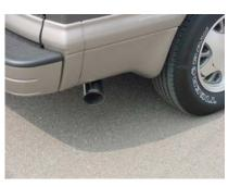
INSTALL YOUR STAINLESS STEEL TIP. USE ANY ALUMINUM OR STAINLESS STEEL CLEANER TO POLISH YOUR TIP. NOW FIRMLY TIGHTEN ALL CLAMPS, HANGERS AND FLANGES.
