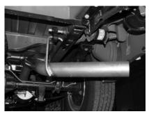
SLIDE OVERAXLE TAILPIPE #E INTO THE OUTLET OF THE MUFFLER 1 ½" TO 2". INSERT WELDED HANGER INTO RUBBER GROMMET AND CLAMP DOWN USING HANGER # D.
