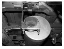
INSTALL REAR MUFFLER HANGER #D ATTACH TO MUFFLER. INSERT WELDED ROD INTO RUBBER GROMMET. THE VERTICAL PART OF THIS HANGER WILL BE ON THE DRIVERS SIDE, DO NOT TIGHTEN.
