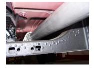
3. Bolt adapter pipe #G to the stock flange re-using the factory clamp. Insert welded hanger into rubber grommet. Do not tighten, just make snug.
