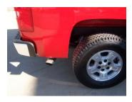
8. Install stainless steel tip. Clamp down. When you have everything in place, firmly tighten all bolts and clamps down securely. Use stainless steel or aluminum cleaner to polish tips. Inspect all fasteners after 25-50 miles of operation and re-tighten as necessary.
