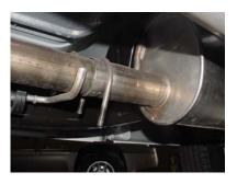
LAY OUT THE EXHAUST ON THE FLOOR SO IT LOOKS LIKE THE DRAWING AND COMPARE PARTS TO THE MANUAL. TO REMOVE THE STOCK EXHAUST UN-CLAMP IT JUST IN FRONT OF THE MUFFLER. YOU MAY NEED TO HEAT IT UP FOR EASIER REMOVAL. LEAVE ALL RUBBER GROMMETS IN PLACE.
