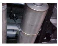
SLIDE BAND CLAMP #H ONTO MUFFLER #B. INSERT HANGERS INTO RUBBER GROMMETS AND ATTACH WITH #I.
