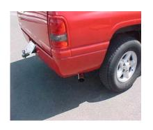
INSTALL STAINLESS STELL TIPS. TO CLEAN STAINLESS TIPS, USE A SCOTCH BRITE PAD AND ANY STAINLESS STEEL OR ALUMINUM CLEANER.
