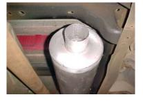
CONNECT MUFFLER #B TO THE FRONT EXTENSION PIPE WITH THE LOUVERS FACING TOWARDS THE CONVERTER. USE A JACK STAND TO SUPPORT THE MUFFLER AND CONNECT WITH CLAMP #E BUT DO NOT TIGHTEN. MUFFLER INLET IS LOOKING INTO THE LOUVERS.
