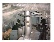
Install the over axle tailpipe # C into the muffler 1-1/2" to 2". Secure to the muffler using clamp # E, do not tighten. Insert welded hangers into rubber grommets on the rear hanger, you will only use one rubber grommet.
