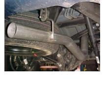
Install stainless tip. Clamp down. When you have everything in place, firmly tighten all bolts and clamp down securely. To clean stainless tip use any stainless cleaner and a scotch brite pad.
