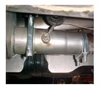
Install head pipe # A on to your existing stock front pipe and secure with clamp # F. Insert welded hanger into rubber grommet. Do not tighten. Install ground strap onto stud on your new head pipe. Use your factory nut.
