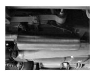
Install muffler #C onto head pipes 1-1/2" to 2" with the louvers facing towards the converter. Use a jack stand to support the muffler. Use clamps #G to secure the muffler to the head pipe. Do not tighten. Muffler inlet is looking into the louvers. Outlets will be on the top.
