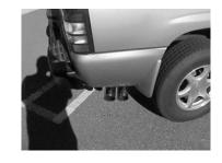
Install rear muffler hanger # H into rubber grommet located just above driverside outlet slide clamp onto muffler outlet.
