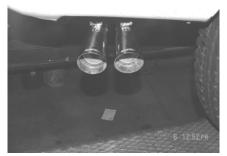
Install stainless steel tips. Clamp down. To clean use a Scott brite pad or any stainless or aluminum cleaner. Now firmly tighten all bolts and clamp down.
