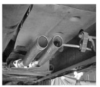
Bolt head pipe #A to the stock head pipe flange behind the converter reusing stock bolts and supplied gasket. Use a Hi-Temperature 02 sensor safe silicone on the gasket for a good seal. Insert welded hanger side into rubber grommet. Reinstall 02 sensor into head pipe. Apply a small amount of anti-seize on the threads. Do not tighten.
