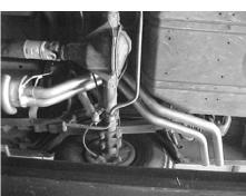
Install the passenger side over axle tailpipe #C onto muffler at least 1-1/2" to 2" using clamp #F to attach tailpipe. Do not tighten. Install Driver side over axle tailpipe #D onto Muffler at least 1-1/2" to 2" using hanger #H to attach tailpipe. Insert into rubber grommet. Use Bolt Kit #I to secure both tailpipes together.
