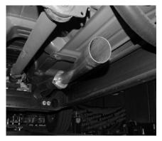
INSTALL HEADPIPE #A ONTO STOCK FLANGE, USE STOCK 15MM NUTS TO SECURE IT. DO NOT TIGHTEN, JUST MAKE SNUG.
