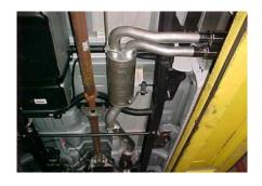
ROTATE THE MUFFLER ASSEMBLY UNTIL THE OUTLETS ARE LEVEL.
