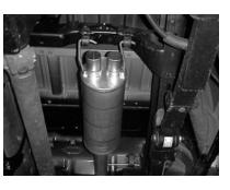
INSTALL MUFFLER #B ONTO HEADPIPE 1-1/2" TO 2" USING CLAMP #J. INSERT WELDED HANGERS INTO RUBBER GROMMET. MAKE SURE OUTLETS ARE LEVEL. USE A JACKSTAND TO SUPPORT MUFFLER. ATTACH HEADPIPE HANGER #K. DO NOT TIGHTEN.
