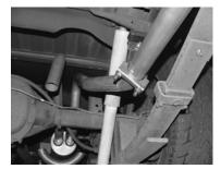
INSTALL PASSENGER SIDE TAILPIPE # C INTO THE MUFFLER 1-1/2" TO 2". ATTACH IT TO THE MUFFLER USING CLAMP # I. THEN USE CLAMP # I TO HOLD TAILPIPE TO HANGER # F. DO NOT TIGHTEN
