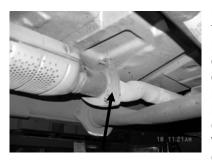
UNBOLT STOCK HEADPIPE AT THE 3 BOLT FLANGE DIRECTLY BEHIND THE CATALYTIC CONVERTER. CUT STOCK TAILPIPE OFF RIGHT BEHIND THE STOCK MUFFLER. LEAVE ALL FACTORY RUBBER GROMMETS IN PLACE. SPRAY WD-40 ON ALL RUBBER GROMMETS FOR EASY REMOVAL.
