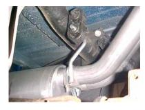
MEASURE 18" FROM THE REAR OF THE FRAME TOWARDS THE FRONT OF THE VEHICLE. USE THIS SLOT FOR THE 10" HANGER #K, INSTALL USING THE 1ST HOLE USE HARDWARE KIT PROVIDED.
