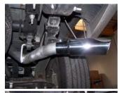
9. NEXT, INSTALL EXIT PIPES #F ONTO TAILPIPES USE CLAMP # J TO
