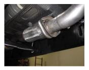
3. Install headpipe #A onto your existing stock 2-bolt flange. Use stock nuts to secure. Do not tighten On short beds cut 12.5" off headpipe
