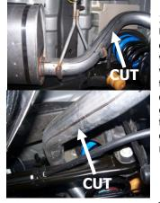
**2.** To remove the stock exhaust, Un clamp it from the clamp in front of the muffler. Do not disguard you will re-use clamp. Disengage the welded hangers using WD-40 from the OEM rubber grommets. Do not damage or remove the rubber grommets as you will reuse them to mount your new system. Now, cut off tailpipe before and after rear axle for removal.
