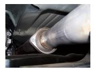
3. Install headpipe #A onto your existing stock front pipe and attach using stock hardware. Do not tighten. Insert welded hanger into rubber grommet.
