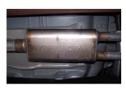
4. Slide muffler #B onto headpipe 1.5-2". Use a jack stand to support the muffler. Use clamp #F to secure the muffler to the headpipe. Do not tighten.
