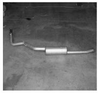
LAY OUT THE GIBSON EXHAUST ON THE FLOOR AND COMPARE PART NUMBERS WITH THE MANUAL. LEAVE ALL FACTORY GROMMETS IN PLACE. FOR EASIER REMOVAL OF GROMMETS AND HANGERS USE WD-40 ON THEM.
