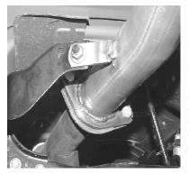
REMOVE THE STOCK EXHAUST BY UNBOLTING THE 17MM BOLTS IN FRONT OF THE MUFFLER. UN-BOLT FACTORY HEADPIPE (YOU WILL RE-USE YOUR FLANGE BOLTS). DO NOT DAMAGE THE FACTORY GASKET YOU WILL NEED TO RE-USE! THEN CUT DIRECTLY BEHIND THE MUFFLER AND REMOVE THE STOCK EXHAUST.
