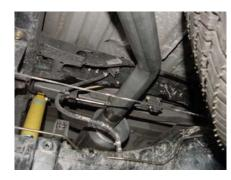
SLIP THE OVER AXLE TAILPIPE #C INTO THE OUTLET OF THE MUFFLER 1" TO 2". CONNECT REAR HANGER WITH FACTORY BOLT. INSERT WELDED HANGER INTO RUBBER GROMMET. USE CLAMP #D TO SECURE TAILPIPE TO THE MUFFLER. DO NOT TIGHTEN.
