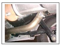
LAY OUT THE GIBSON EXHAUST ON THE FLOOR AND COMPARE PART #'S TO THE DRAWING. TO REMOVE YOUR FACTORY EXHAUST UN-BOLT YOUR TAILPIPE AT THE CLAMP LOCATED BEHIND YOUR STOCK MUFFLER USE WD-40 TO AID YOU IN REMOVAL OF HANGERS FROM RUBBER CDUMMETS
