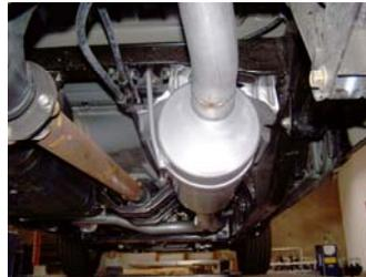
6. Slide muffler #C onto the resonator 1.5-2". Use clamp #G to secure muffler to resonator. Do not tighten. Outlet will be at the 12 o'clock position. Inlet of muffler will be looking into the louvers.
