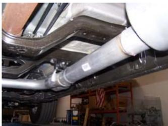
5. Slide resonator #B onto the Y Pipe 1 1/2"-2". Use clamp #G to secure pipes together. Do not tighten.
