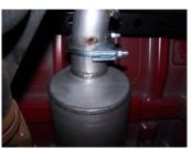
4. Install muffler #B onto headpipe 11/2"-2" with the louvers facing towards the converter. Use a jack stand to support the muffler. Use clamp #E to secure the muffler to the headpipe. DO NOT TIGHTEN. Muffler inlet is looking into the louvers. Outlet of muffler will be at approximately 12 o'clock.
