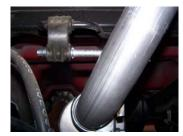
5. Install tailpipe #C into muffler approximately 1½-2". Secure tailpipe with clamp #E. DO NOT TIGHTEN. Insert welded hanger into rubber grommet.
