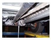
2. Bolt head pipe #A onto your existing stock front pipe and attach with factory hardware. DO NOT TIGHTEN. Use a jack stand to support the converter. Insert welded hangers into rubber grommet.
