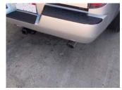
**5.** Install stainless steel tips #D. Clamp down. When you have everything in place, firmly tighten all bolts and clamps down securely. Use stainless steel cleaner and a Scotch Brite pad weekly to prevent tip from discoloration.
