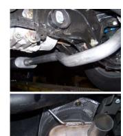
**4.** Install tailpipe and resonator assembly #C into muffler 1½"-2". Use clamp #E to secure to muffler. DO NOT TIGHTEN. Insert welded hangers into rubber grommets.
