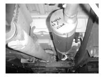
INSTALL REAR MUFFLER HANGER #E INTO RUBBER GROMMET. THE CLAMP WILL BE USED TO SECURE THE TAILPIPE TO THE MUFFLER, DO NOT TIGHTEN.
