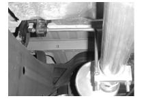
NSTALL MUFFLER #B ONTO HEADPIPE 1-1/2" TO 2" WITH INLET TOWARDS THE ENGINE. OUTLET SHOULD BE AT THE 2 O'CLOCK POSITION. USE CLAMP #E AND #F TO SECURE MUFFLER TO THE HEADPIPE, INSERT MUFFLER HANGER INTO RUBBER GROMMET. DO NOT TIGHTEN. THE INLET OF THE MUFFLER IS
