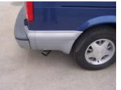
INSTALL STAINLESS STEEL TIP, CLAMP DOWN. NOW TIGHTEN ALL BOLTS AND CLAMPS. TO CLEAN TIP US SCOTCH BRITE AND ANY STAINLESS OR ALUMINIUM CLEANER.
