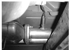
RE-INSTALL O2 SENSOR. USE A SMALL AMOUNT ANTI-SIEZE ON THE THREADS. NOW FIRMLY TIGHTEN ALL CLAMPS, HANGERS, FLANGE, AND BOLTS.
