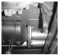
REMOVE O2 SENSOR FROM STOCK HEAD PIPE AND UN-BOLT STOCK HEADPIPE. YOU WILL REUSE YOUR STOCK NUTS AND BOLTS. CUT STOCK EXHAUST JUST BEHIND THE MUFFLER FOR EASIER REMOVAL. LEAVE ALL RUBBER GROMMETS IN PLACE. FOR EASIER REMOVAL OF HANGERS SPRAY WD-40 TO AID YOU IN REMOVING THEM. BOLT HEADPIPE #A TO STOCK FLANGE USING SUPPLIED FLANGE GASKET #I AND REUSING FACTORY BOLTS. APPLY A SMALL A MOUNT OF HIGH-TEMP O2 SENSOR SAFE SILICONE ON THE FLANGE TO PREVENT ANY LEAKS.
