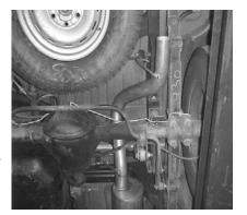
INSTALL THE OVERAXLE TAILPIPE #C INTO MUFFLER AT LEAST 1 1/2" TO 2" USING CLAMP #F. DO NOT TIGHTEN. INSERT WELDED HANGERS INTO RUBBER GROMMETS. THE SPARE TIRE ON SOME VEHICLES MAY NEED TO BE LOOSENED AND PULLED TO THE DRIVER SIDE AND RE-TIGHTENED. ROTATE PIPES UNTIL YOU HAVE AT LEAST A 1" CLEARANCE AWAY FROM ALL PIPES, ETC.
