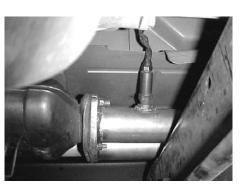
RE-INSTALL O2 SENSOR. USE A SMALL AMOUNT ANTI-SIEZE ON THE THREADS. NOW FIRMLY TIGHTEN ALL CLAMPS, HANGERS, FLANGE, AND BOLTS.
