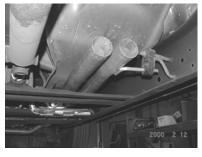
BOLT HEADPIPE #A USING SUPPLIED FLANGE GASKET #G AND REUSING FACTORY BOLTS. APPLY A SMALL A MOUNT OF HIGH-TEMP O2 SENSOR SAFE SILICONE ON THE FLANGE TO PREVENT ANY LEAKS. INSERT WELDED HANGER INTO RUBBER GROMMET. DO NOT TIGHTEN
