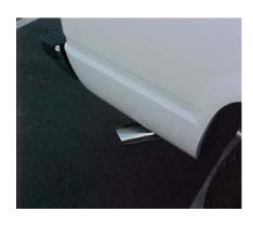
INSTALL TURNOUT PIPE #D INTO TAILPIPE USING CLAMP #G . INSTALL THE STAINLESS TIP AND CLAMP DOWN. USE ANY STAINLESS STEEL OR ALUMINUM CLEANER TO POLISH TIP. TIGHTEN ALL NUTS ,BOLTS AND CLAMPS.
