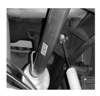
SLIDE MUFFLER WITH DUAL INLET ONTO HEADPIPE AT LEAST 1-1/2" TO 2". MUFFLER OUTLET SHOULD BE AT THE 12 O'CLOCK POSITION. USE CLAMPS #F TO ATTACH TO THE HEADPIPE. MAKE SURE INLETS AND MUFFLER IS LEVEL. AND TIGHTEN DOWN. USE JACK STAND TO SUPPORT MUFFLER.
