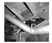
**INSTALL THE OVERAXLE** TAILPIPE #C INTO MUFFLER AT LEAST 1 1/2" TO 2" USING CLAMP #G. DO NOT TIGHTEN. INSERT WELDED HANGERS INTO RUBBER GROMMETS. THE SPARE TIRE ON SOME VEHICLES MAY NEED TO BE LOOSEN ED AND PULLED TO THE DRIVER SIDE AND RE-TIGHTENED. ROTATE PIPES UNTIL YOU HAVE AT LEAST A 1" CLEARANCE AWAY FROM SHOCK, BRAKE LINES, SPARE TIRE, ECT.
