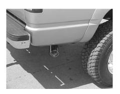
INSTALL STAINLESS STEEL TIP. TO CLEAN YOUR TIP USE ANY STAINLESS OR ALUMINUM CLEANER. TIGHTEN ALL CLAMPS, HANGERS AND CHECK FOR LEAKS.
