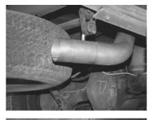
INSTALL TURNOUT #D PIPE ONTO TAILPIPE. ROTATE PIPE TILL IT IS LEVEL. USE CLAMP #F TO SECURE PIPE. DO NOT TIGHTEN.
