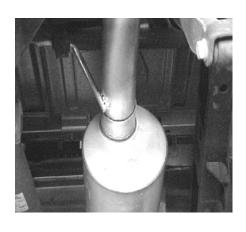
NEXT CONNECT THE MUFFLER TO THE HEADPIPE USING CLAMP #E. USE JACKSTANDS TO SUPPORT THE MUFFLER. THE OUTLET OF THE MUFFLER WILL BE AT APPROXIMATELY 11 O'CLOCK. THE MUFFLER INLET IS LOOKING INTO THE LOUVERS.
