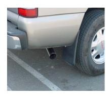
INSTALL THE STAINLESS STEEL TIP NOW, FIRMLY TIGHTEN EVERYTHING ALL CLAMP, HANGERS, BOLTS, FLANGE. TO CLEAN TIP USE ANY STAINLESS CLEANER WITH A SCOTCH BRITE PAD.
