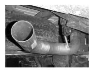
Install exit pipe #D onto the tailpipe. Insert welded hanger into rubber grommet. Secure pipes together with clamp # E. Do not tighten. Roll the exit pipe until it is at the correct angle for your truck.
