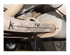
TO REMOVE YOUR STOCK EXHAUST, MEASURE 16" FROM THE MUFFLER FORWARD TOWARDS THE FRONT OF THE VEHICLE. LEAVE ALL RUBBER GROMMETS ON THE HANGER. USE WD-40 TO AID IN THE REMOVAL OF THE EXHAUST AND HANGERS
