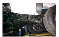
INSTALL EXIT PIPE #E ONTO TAILPIPE. INSERT WELDED HANGER INTO RUBBER GROMMET. USE CLAMP #H TO SECURE THE EXIT PIPE TO THE TAILPIPE. DO NOT TIGHTEN. ROTATE THE PIPE UNTIL IT IS LEVEL.
