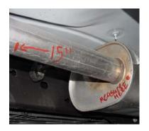
TO REMOVE STOCK EXHAUST MEASURE 4" FROM THE FRONT OF THE MUFFLER FORWARD AND CUT. NOW CUT OFF YOUR STOCK TAILPIPE JUST BEHIND THE MUFFLER AND REMOVE. LEAVE ALL RUBBER GROMMETS ON THE HANGER. USE WD-40 TO AID IN THE REMOVAL OF THE EXHAUST AND HANGERS.
