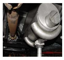
NEXT INSTALL MUFFLER #C. SLIDE IT ONTO HEADPIPE 1-1/2" TO 2". AND ATTACH USING CLAMPS # F. INLET OF MUFFLER SHOULD FACE TOWARDS THE MOTOR. MUFFLER INLET IS LOOKING INTO THE LOUVERS.
