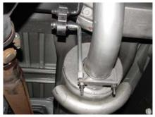
INSTALL REAR MUFFLER HANGER #G INTO RUBBER GROMMET LOCATED JUST ABOVE THE OUTLET OF THE MUFFLER. SLIDE CLAMP ONTO MUFFLER OUTLET. DO NOT TIGHTEN.
