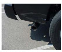
INSTALL YOUR STAINLESS STEEL TIPS. TO CLEAN TIPS USE ANY STAINLESS OR ALUMINUM CLEANER AND A SCOTCH BRITE PAD. NOW TIGHTEN ALL NUTS, BOLTS AND CLAMPS STARTING FROM THE FRONT AND WORKING BACK.
