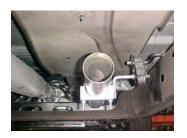
Install head pipe #A onto your existing 2-bolt flange using your factory bolts. Do not tighten. Next slide front hanger # G onto head pipe. Insert hanger into rubber grommet. Do not tighten
