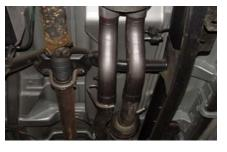
SLIDE PASSENGER SIDE HEADPIPE #A ONTO STOCK HEADPIPE. INSERT WELDED HANGER INTO RUBBER GROMMET. NEXT INSTALL DRIVERS SIDE HEADPIPE #B ONTO STOCK HEADPIPE, USE CLAMP #G TO SECURE BOTH HEADPIPES, DO NOT TIGHTEN.
