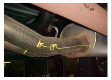
TO REMOVE STOCK EXHAUST, CUT 13" FROM THE FRONT OF THE MUFFLER,
