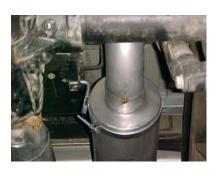
SLIDE MUFFLER #C ONTO HEADPIPES 1-1/2" TO 2". USE A JACK STAND TO SUPPORT MUFFLER.
