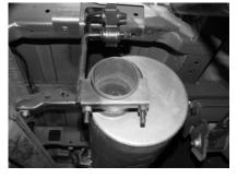
INSTALL REAR MUFFLER HANGER #D ATTACH TO MUFFLER. INSERT WELDED ROD INTO RUBBER GROMMET. THE VERTICAL PART OF THIS HANGER WILL BE ON THE DRIVERS SIDE, DO NOT TIGHTEN.
