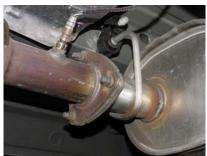
TO REMOVE STOCK EXHAUST UNBOLT IT FROM THE 3-BOLT FLANGE LOCATED JUST BEHIND THE CATALYTIC CONVERTER. YOU WILL REUSE YOUR FACTORY BOLTS. NOW CUT OFF YOUR STOCK TAILPIPE JUST BEHIND THE MUFFLER AND REMOVE. LEAVE FACTORY RUBBER GROMMETS IN PLACE. USE WD-40 TO AID IN REMOVAL OF EXHAUST AND HANGERS.
