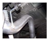
NEXT, INSTALL OVERAXLE TAILPIPE # D INTO MUFFLER 1-1/2"- 2". USE CLAMP # I TO SECURE PIPE TO MUFFLER, DO NOT TIGHTEN. INSERT HANGER INTO RUBBER GROMMET.
