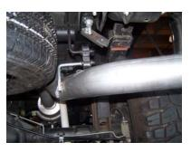
SLIDE EXIT PIPE # E ONTO OVERAXLE TAILPIPE INSERT WELDED HANGER INTO RUBBER GROMMET. USE CLAMP # I TO SECURE PIPES TOGETHER. DO NOT TIGHTEN. ROTATE PIPE UNTIL LEVEL.
