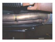
TO REMOVE STOCK EXHAUST, CUT 13" FROM THE FRONT OF THE MUFFLER. MEASURE TOWARDS THE FRONT OF THE VEHICLE. LEAVE ALL RUBBER GROMMETS ON THE HANGER. USE WD-40 TO AID IN THE REMOVAL OF EXHAUST AND HANGERS. SUPPORT THE CATALYTIC CONVERTER BEFORE CUTTING.
