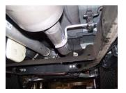
2. Bolt head pipe #A onto your existing stock front pipe re-using stock nuts/bolts. Insert welded hanger into rubber grommet. DO NOT TIGHTEN.
