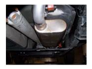
**4.** Install muffler onto head pipe #A.  $1\frac{1}{2}$ "-2" with the louvers facing towards the converter. Use a jack stand to support the muffler. Use clamp #E to secure the muffler to the headpipe. DO NOT TIGHTEN. Muffler inlet is looking into the louvers. Outlet will be on the drivers side.
