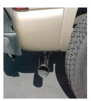
**11.** Install stainless steel tips. Clamp down. When you have everything in place, firmly tighten all bolts and clamps down securely. Use stainless steel cleaner and a Scotch Brite pad weekly to prevent tip from discoloration. Inspect all fasteners after 25-50 miles of operation and re-tighten as necessary.
