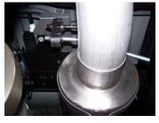
**4.** Slide muffler #B onto head pipe #A 1½"-2". Use a jack stand to support the muffler. Use band clamp #G to secure the muffler to the head pipe, slide hanger on band clamp into rubber grommet. Do not tighten.
