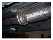
2. Remove the stock exhaust by unbolting it at the clamp located in front of the muffler. Disengage the welded hangers from the OEM rubber grommets. Use WD-40 to aid in this process. Do not damage stock nuts and bolts or remove the rubber grommets as you will re-use them to mount your new system. Now, cut off tailpipe and remove system.
