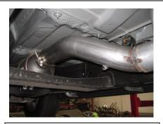
1.Install headpipe #A onto your factory pipe using your stock clamp insert welded hanger into the rubber grommet leave clamp loose.
