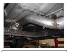
1.Install headpipe #A onto your factory pipe using your stock clamp insert welded hanger into the rubber grommet leave clamp loose.
