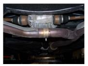
2. First, remove the stock exhaust. Remove the clamp on the driver side pipe in the center of the vehicle. Then cut just before the factory Y-pipe. (See pictures) Disengage the welded hangers. Use WD-40 to aid in this process. Do not remove the rubber grommets as you will reuse them to mount the new system. Now remove the exhaust system.
