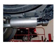
4. Install passenger side muffler assembly #C onto Y-pipe. Insert welded hangers into rubber grommets. Use clamp #D to secure assembly to Y-pipe. Do not tighten.
