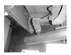
Slide turn out pipe #D on the tailpipe behind the rear tire, & hook to your existing hanger. Roll turnout pipe until you have it at the correct angle for your truck and connect with clamp #F.
