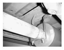
Remove & cut stock exhaust at the first connection approximately 12" in front of your stock muffler. Use jack stands to support converter.
