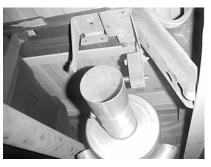
Slide muffler #A with inlet towards the converter onto your stock front extension pipe. Use a jack stand to support the muffler and connect with hanger #G but do not tighten. Muffler inlet is looking into the louvers.
