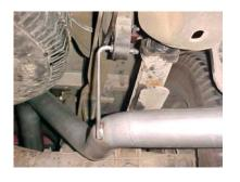
NEXT, INSTALL REAR MUFFLER HANGER #G ONTO TAILPIPE. INSERT HANGERS INTO RUBBER GROMMET.
