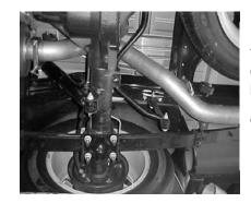
INSTALL OVERAXLE TAILPIPE #B AND CONNECT TO THE MUFFLER USING HANGER # G. INSERT WELDED HANGER INTO RUBBER GROMMETS.
